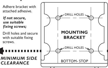
Adhere bracket with attached adhesive.
